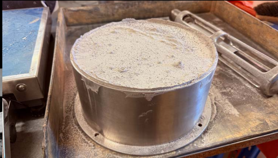
Stainless steel container with LHS-1
