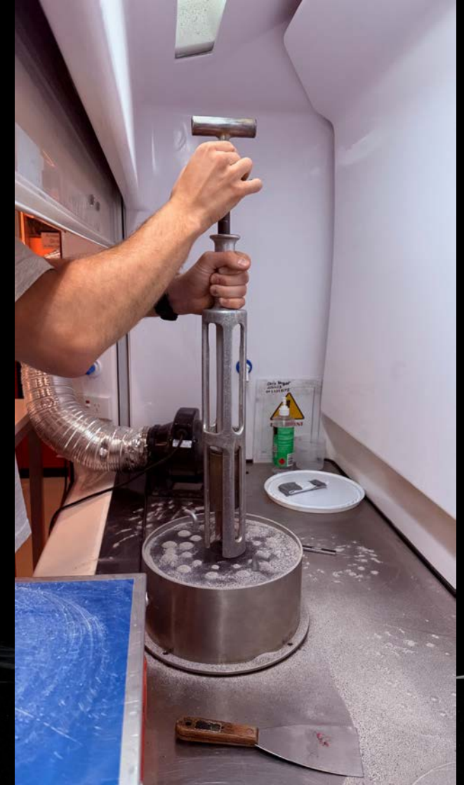
Plate compaction with Proctor hammer
